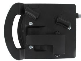
Designed for motor home and fifth wheel trailer entrance doors, this new product is a redesign of our 030-1000/030-1050 Motor Home Entrance Door Hardware. It features easy installation through sandwich mounting, a reliable direct release rotary latch which is compliant to FMVSS 206 (ECE R11), a builtin deadbolt for additional security and is power lockable.
